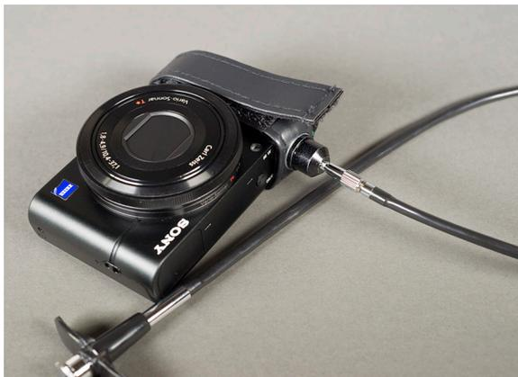
Figure A-9: Hama Cable Release Attached to RX100
