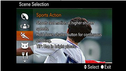
Figure 3-26: Help Screen for Scene Mode Setting
