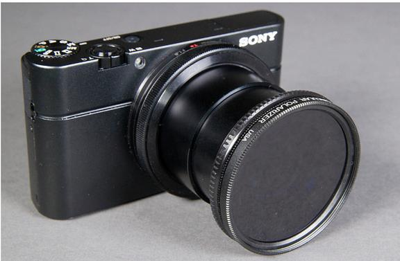
Figure A-6: *Circular Polarizer Attached with Lensmate Adapter*
