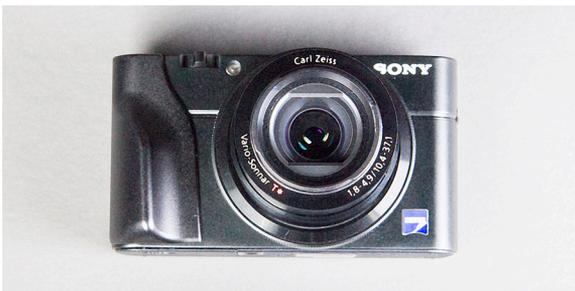
Figure A-7: Custom-made Grip on Front of RX100
