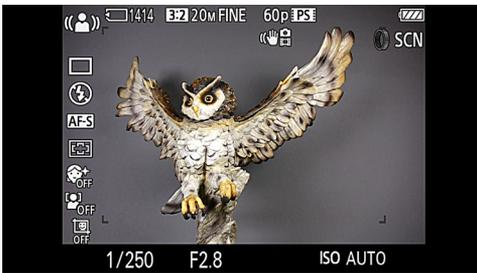
Figure 3-25: Shooting Display with Anti Motion Blur Setting
