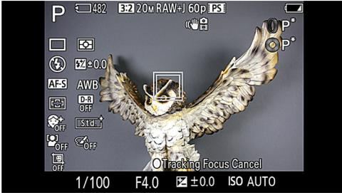
Figure 2-19: Tracking Focus in Use
