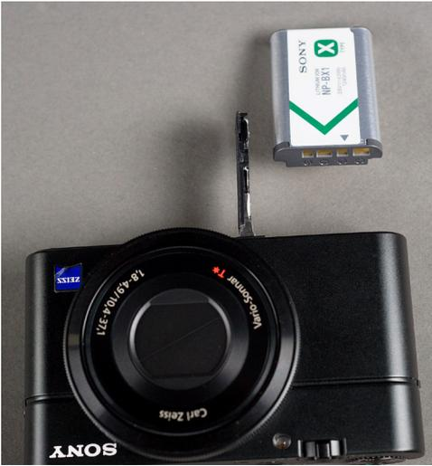
Figure 1-1: Battery lined up for insertion into RX100
