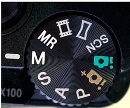
Figure 3-21: Manual Exposure Mode
