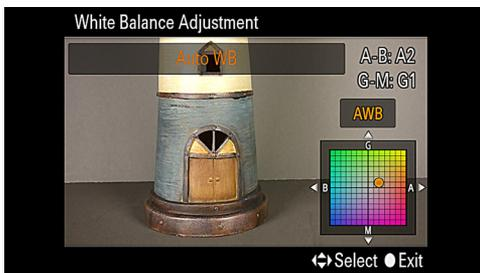
Figure 4-56: White Balance Adjustment Screen
