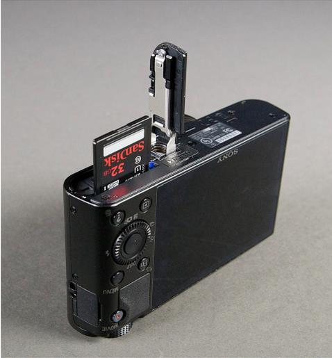
Figure 1-9: Inserting SD Card into RX100
