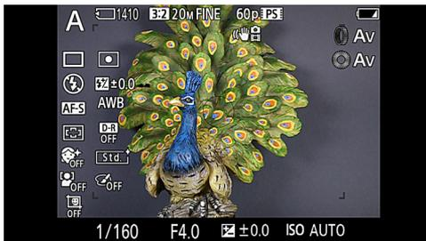
Figure 5-10: Icons Show Two Controls for Aperture
