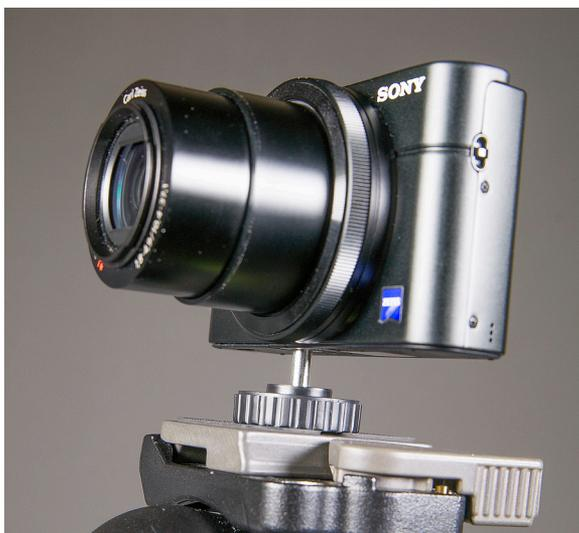
Figure A-21: RX100 with Tripod Screw Attached to Tripod
