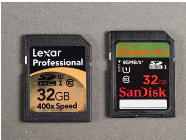
Figure 1-7: High-Speed SDHC Cards
