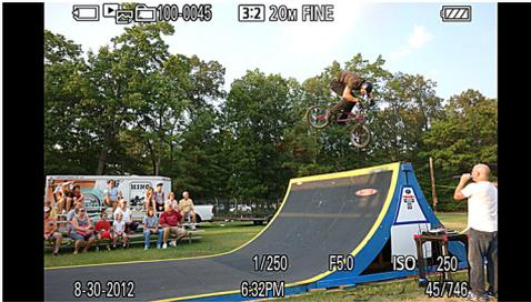
Figure 6-5: Playback Display with Basic Information
