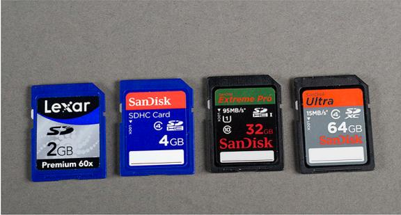
Figure 1-4: Card Types: SD, SDHC, SDHC 32GB, SDXC
