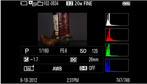
Figure 6-7: Histogram for Dark Image, with Peaks at Left
