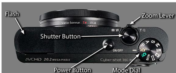
Figure 5-1: Controls on Top of Camera
