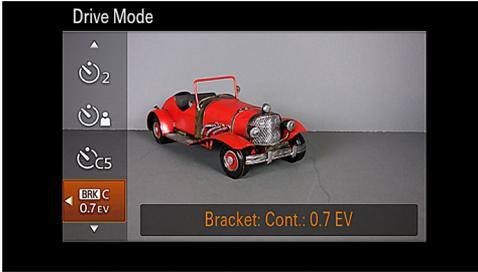
Figure 4-18: Drive Mode - Exposure Bracketing
